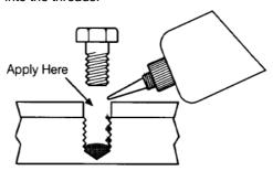
**7.** Assemble and tighten as usual. When tightening to established torque values, torque compensation is not required.
